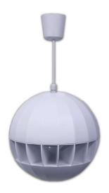
PS820 is the right choice for installations at high ceiling areas without columns, such as warehouses, hypermarkets and large showrooms that require even sound distributions. It is built with 8" speaker of 20W 100V rating, delivering powerful and evenly projected sound with 360° dispersion.
