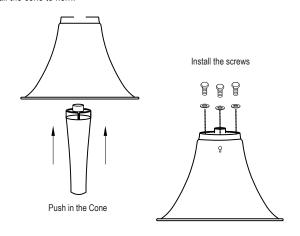
3: Install the bracket to the horn flare assembly.
