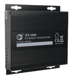
**iPX5400** works in a pair, and is convenient way of sending audio and RS485 data to another location through LAN, dedicated fiber or network cable. In the case of using dedicated fiber link, an Ethernet to fiber converter shall be required.
