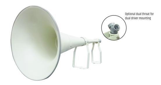
**LH201** is a long throw horn speaker with 21" round flare, made from solid aluminium housing for a solid sound throw. It is suitable for outdoor installation with stainless steel fasteners and powder epoxy coated steel brackets.
