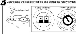
Connect the speaker cable from the ceiling to the connectors provided. Ensure polarity of cable is correctly terminated to the terminals. Pre-select the power output required to suit the installation area before mounting the speaker to the ceiling.
