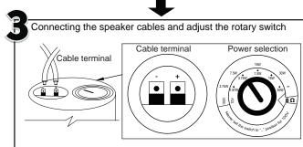
Connect the speaker cable from the ceiling to the connectors provided. Ensure polarity of cable is correctly terminated to the terminals. Pre-select the power output required to suit the installation area before mounting the speaker to the ceiling.
