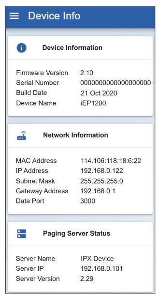
Note: If Paging Server IP address is changed to an unknown value, turn On the Auto Connect allow iEP1200 auto capture the server IP address and show up in the device information page.
