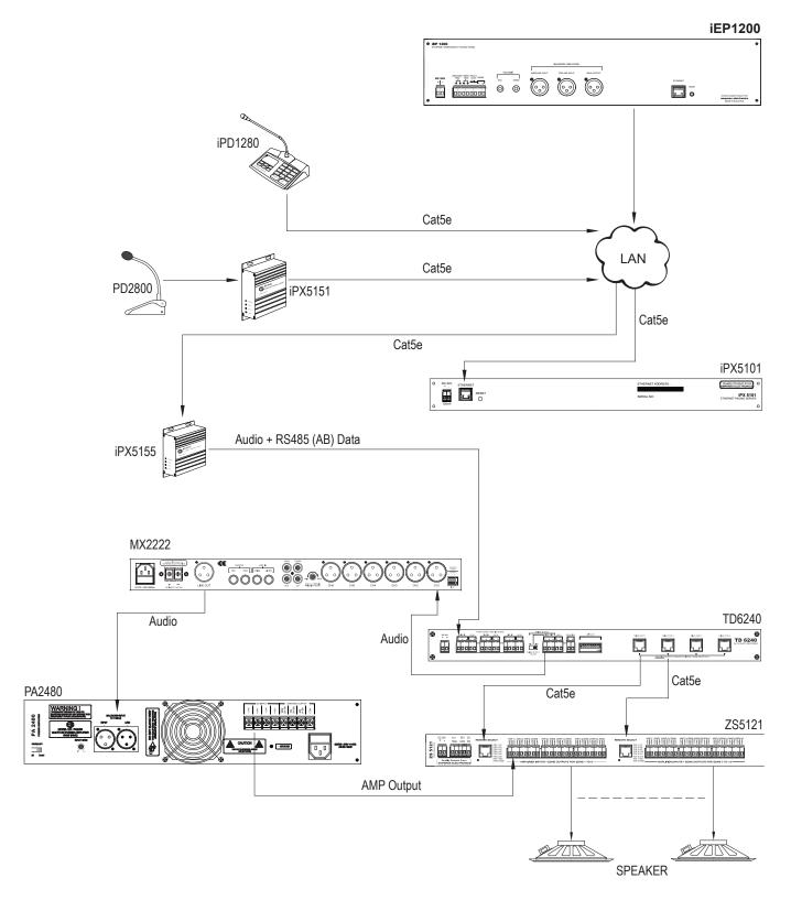
iEP1200, which is installed at main rack for a large system using IP as communication interface, shall be able to override remote buildings / system as similar to single rack installation.
