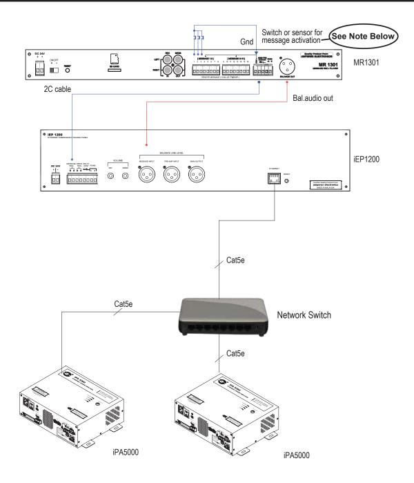
The dry contact at the MR1301 is used to trigger iEP1200, thus overriding the normal audio source for priority paging. It is then connected to the Emergency Relay trigger at the Zone Selector, providing a dry contact for connecting 24V DC to override external volume controllers.
