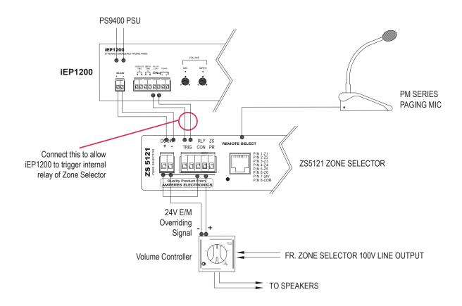
The above diagram shows detailed connections for using iEP1200 to override volume control and activating ALL CALL at zone selector.
